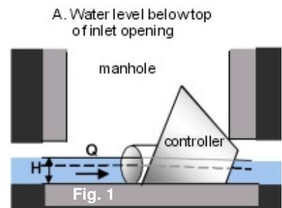
When it starts raining the feed flow increases and the water level in front of the regulator increases. When the water's surface is above the top of the regulator's intake opening, but is still below the top of the controller vortex chamber, air is trapped inside the vortex chamber, and the flow's cross section is reduced. This increased resistance limits the water's flow through the regulator (Fig. 2).
