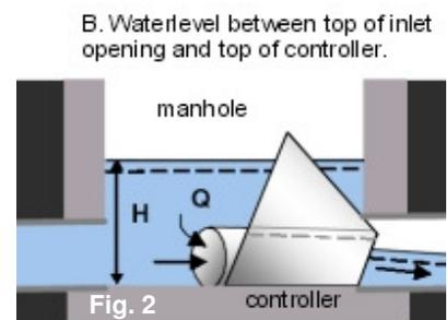
When the water's surface in front of the flow regulator rises above the top of the vortex chamber, the head will make the water in the regulator rotate. The trapped air forms a core in the vortex valve and the flow's cross section is heavily reduced at the outlet. The result is a considerable pressure loss, as intended (Fig. 3).
