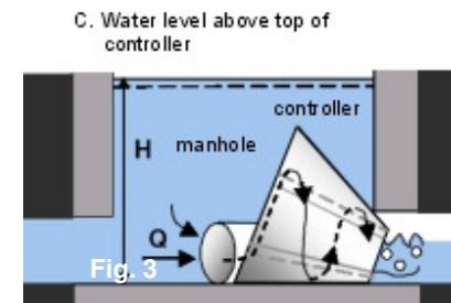
After the rain stops the feed flow decreases. The water level in the structure eventually falls below the top of the vortex chamber and the dropping pressure causes the rotation to stop. Air is drawn into the vortex chamber - with some delay - hence the hysteresis in the head-discharge curve (Fig. 4).
